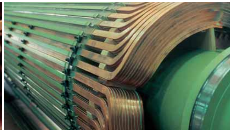
AC generator, Alstom (CH)
