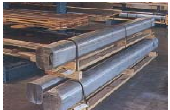
Billet awaits shipment to a nearby forge shop at the Haynes International service center in La Mirada, California.
