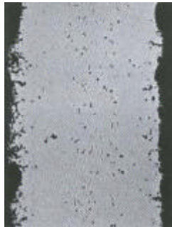
230 alloy Average Metal Affected = 5.2 Mils (132 µm)/Side
