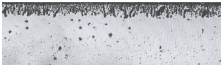
INCONEL alloy 601 Average Metal Affected = 5.3 mils (135 µm)
