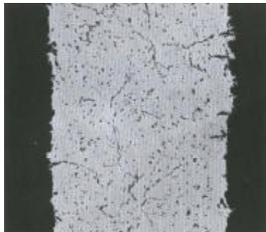
HASTELLOY X alloy Average Metal Affected = 12.9 Mils (328 µm)/Side
