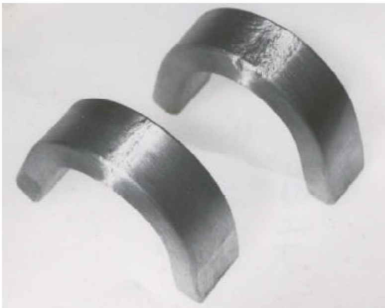
Typical face and root bends for welded 230® alloy 0.5-inch (13 mm) plate and matching filler metal. Bend radius was 1.0-inch (25 mm).
