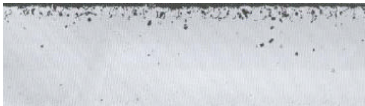
230 alloy Average Metal Affected = 3.4 mils (86 µm)
