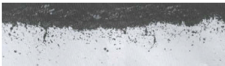
Alloy 800H Average Metal Affected = 8.9 mils (226 µm)
