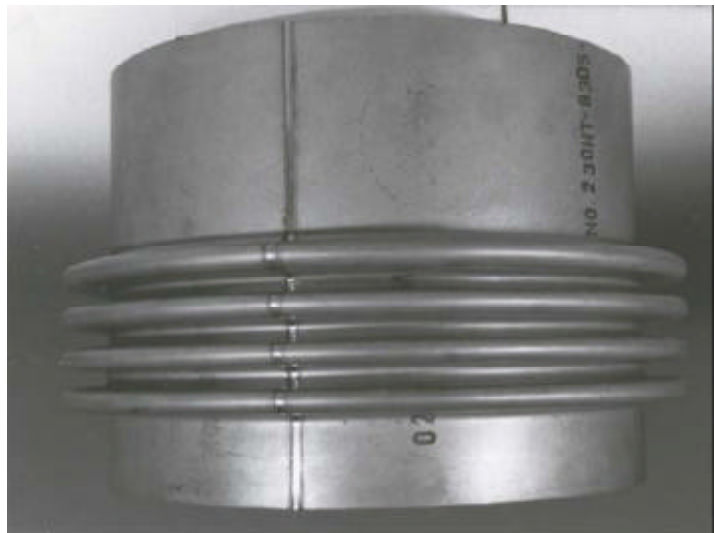
Prototype 230 high-temperature expansion bellows made of 0.020-inch (0.5mm) thick sheet in a catalytic cracker configuration.
