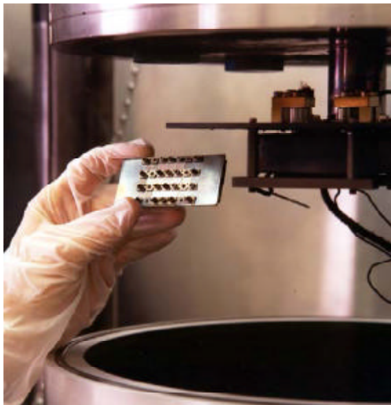
Substrate holder and box of 230 alloy resist temperatures of 1650°F (899°C) during the production of semiconductors.
