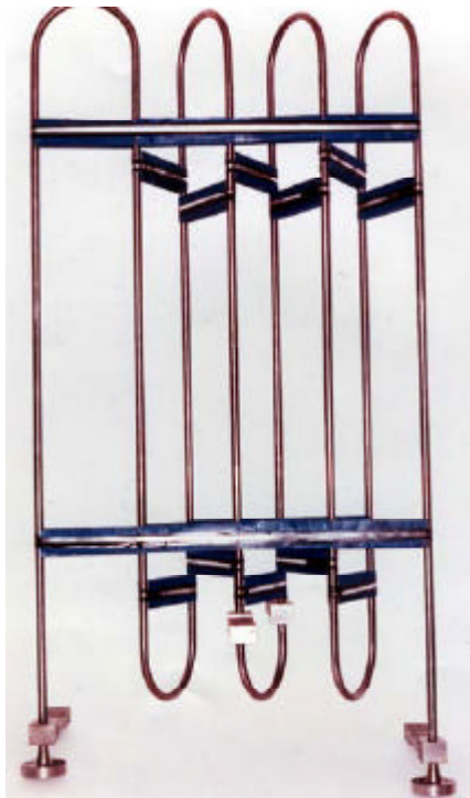
Resistance-heated 230 superheater tubes at the Penn State Applied Research Laboratory. Used to produce about 1625°F (885°C) high-pressure steam.
