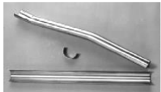
HR-160 tube shields are considered the premier superheater tube shield material for municipal and industrial waste incineration systems. The use of HR-160 alloy has resulted in greatly improved life in municipal waste incinerators where high temperature corrosion and fly ash erosion are major considerations.
